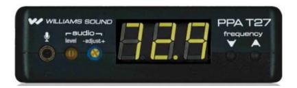
In our experience attaching the Mic 044 to this jack results in the level indicator not flashing even if the gain is turned up all the way. The audio heard on the receivers is weak and hard to hear.
